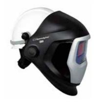
$3M^{\mathbb{M}}$  Speedglas<sup> $\mathbb{M}$ </sup> Welding Helmet 9100 with safety helmet adapter and  $3M^{\mathbb{M}}$  Peltor<sup> $\mathbb{M}$ </sup> Safety Helmet G3001. A Uvicator is built into the G3001 helmet. When the helmet is new the Uvicator is red, as UV-radiation takes its toll on the plastic, the red Uvicator gradually fades out. When the red has faded away completely, it is time to replace the helmet.
